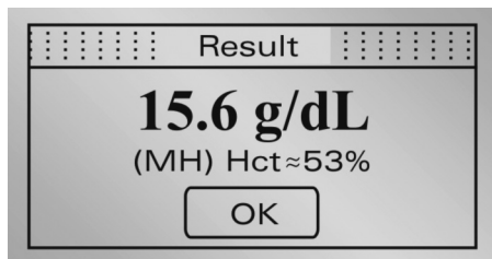
Patient Types: M ... Male, F ... Female, C ... Child Symbols for exceeding Hgb-limits: H ... Result above upper limit threshold L ... Result below lower limit threshold Illustration 22: Display showing the test result.
