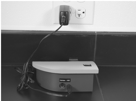
Illustration 3: Connecting the power adaptor.
