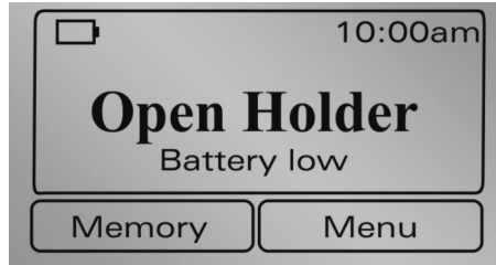
Illustration 34: Display screen when battery is discharged.
