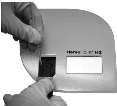
Illustration 32: Removing the Alere HemoPoint® H2 Microcuvette holder.
