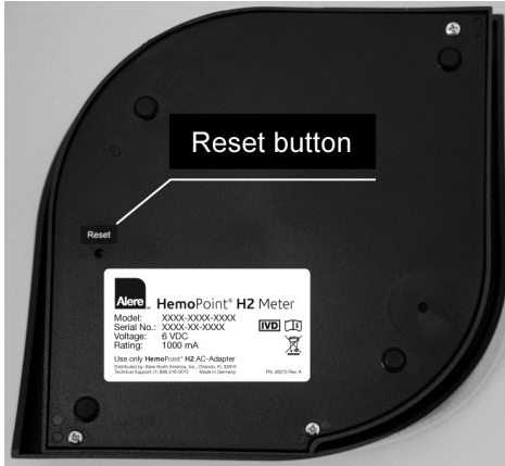
Illustration 35: Location of the reset button.
